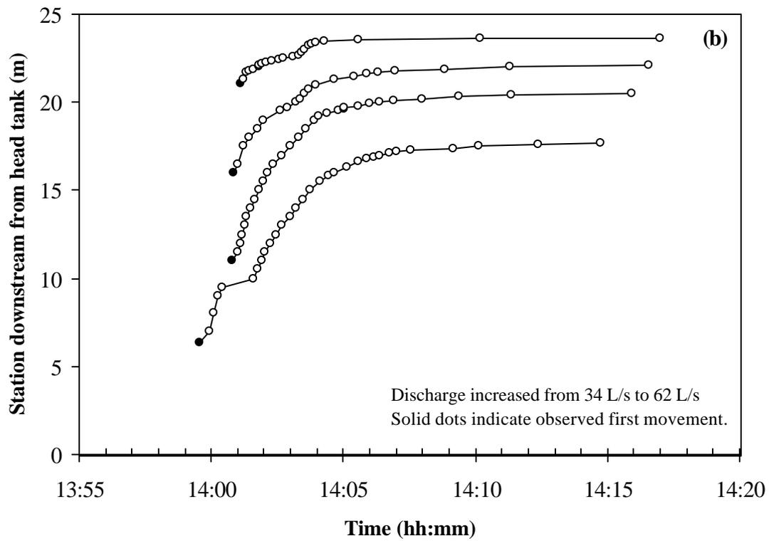
**Figure 8. Propagation of tracking particles placed on the surface of the initial accumulation following (a) 30% increase and (b) 85% increase in discharge.**
