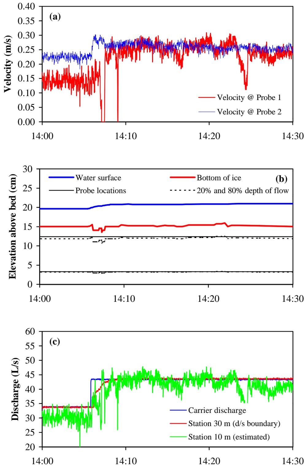
**Figure 10. Test 1 - Continuous velocity, depth, ice thickness, and estimated discharge at station 10m.**
