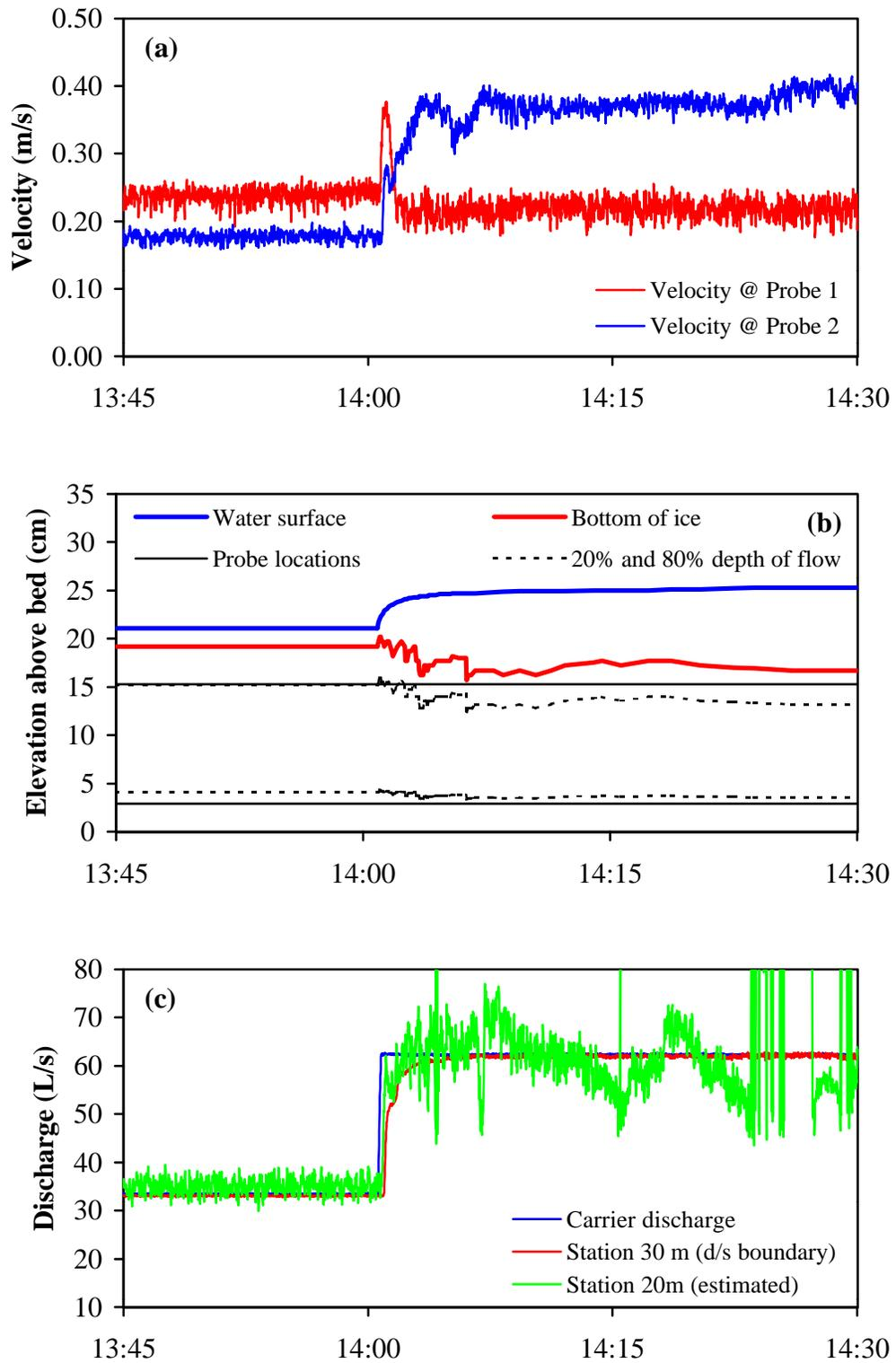
**Figure 13. Test 2 - Continuous velocity, depth, ice thickness, and estimated discharge at station 20m.**
