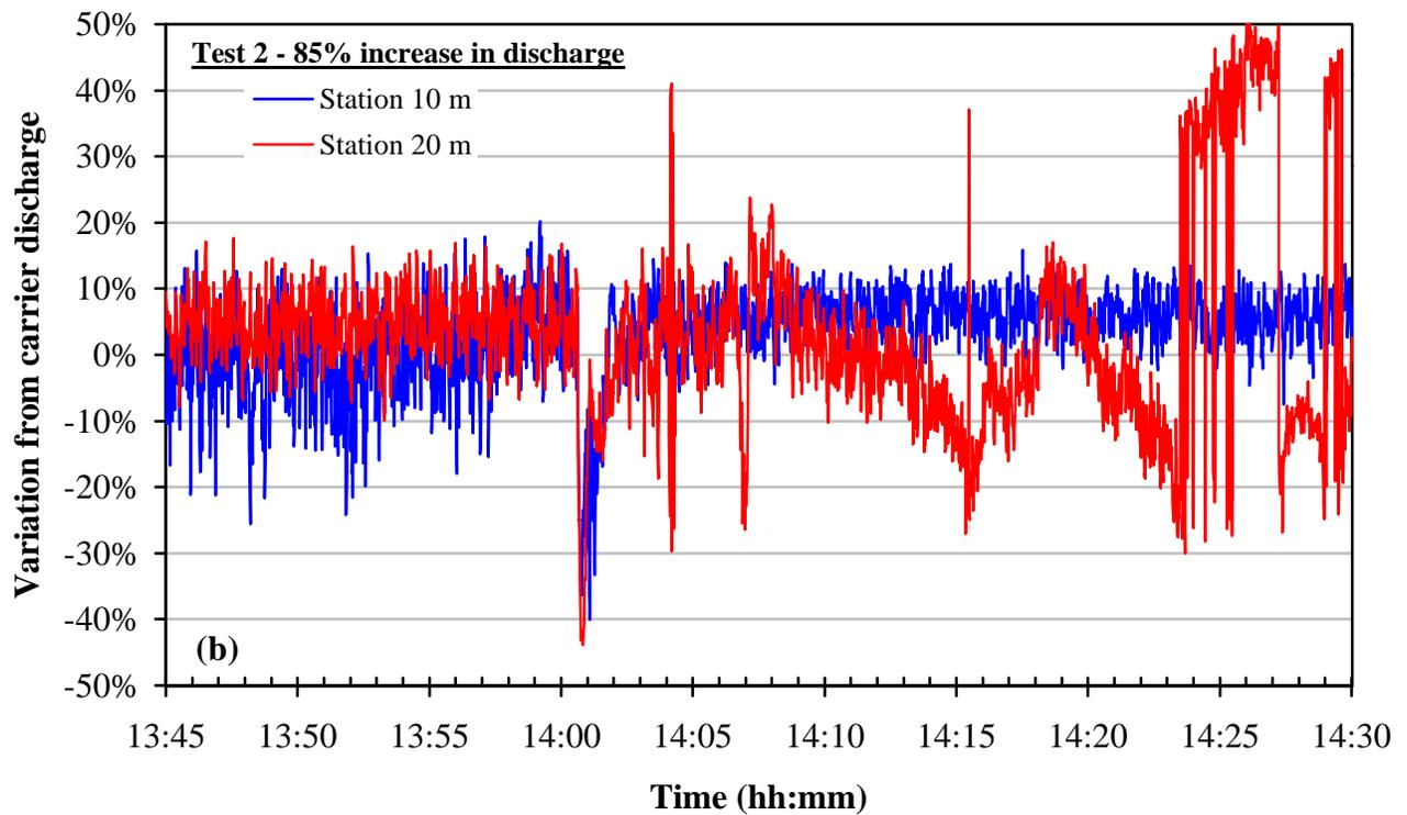
**Figure 14. Variation of estimated discharge at stations 10 and 20 m from carrier discharge for (a) 30% increase in discharge and (b) 85% increase in discharge.**
