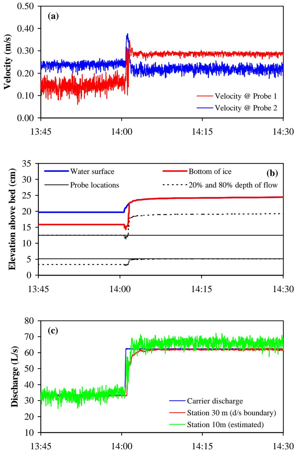
**Figure 12. Test 2 - Continuous velocity, depth, ice thickness, and estimated discharge at station 10m.**
