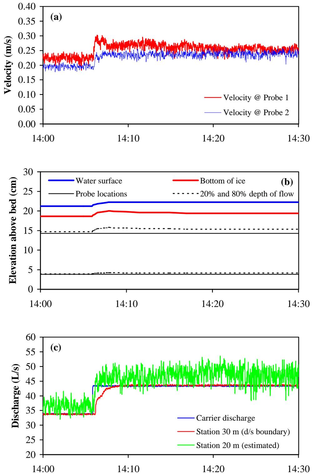
**Figure 11. Test 1 - Continuous velocity, depth, ice thickness, and estimated discharge at station 20m.**
