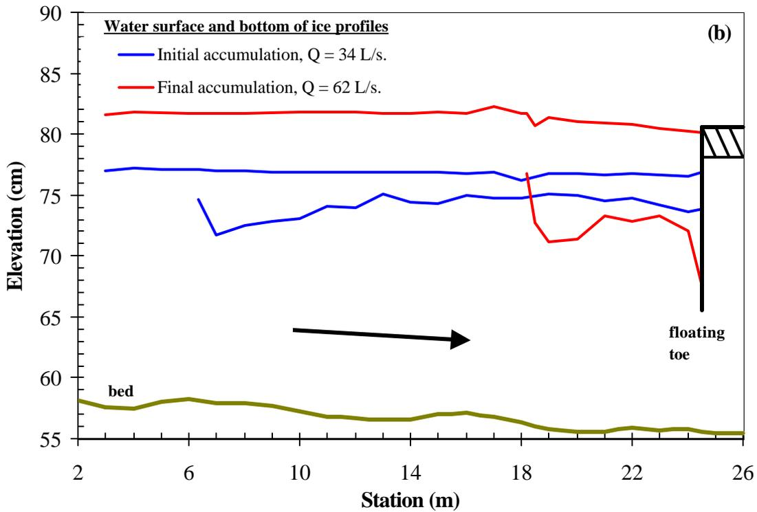
**Figure 9. Water surface and bottom of ice profiles for initial and final accumulations for (a) 30% increase in discharge and (b) 85% increase in discharge.**
