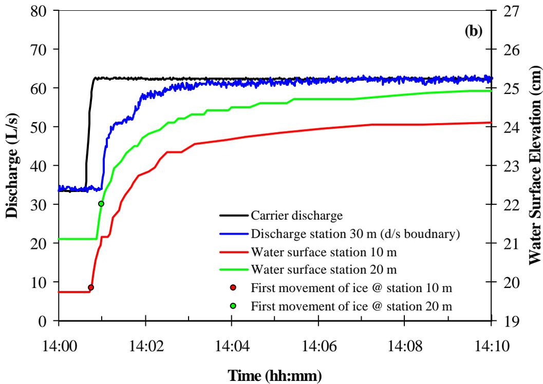
Figure 7. Continuous discharges and observed water levels during shoving of ice accumulation for (a) 30% increase in discharge and (b) 85% increase in discharge.
