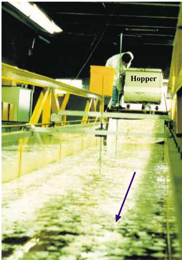
**Figure 4. Loading ice for initial accumulation.**
