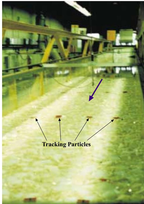
**Figure 5. Placement of tracking particles on surface of initial accumulation.**
