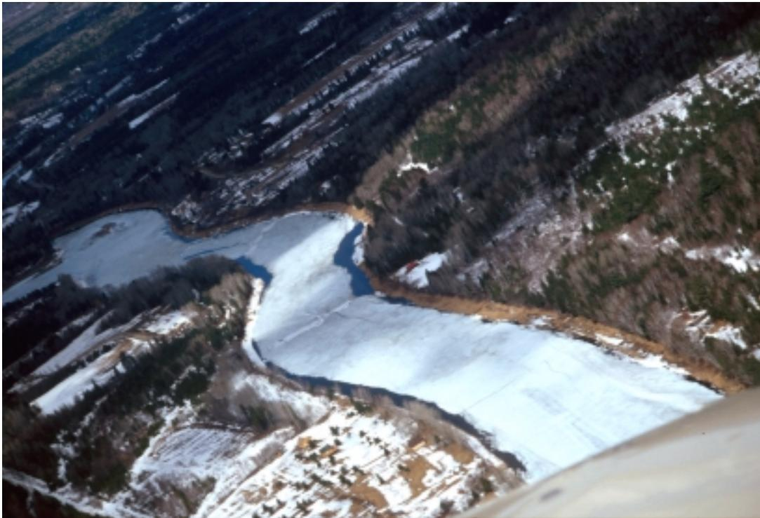
Fig. 6. Aerial view of river illustrating transverse cracks
