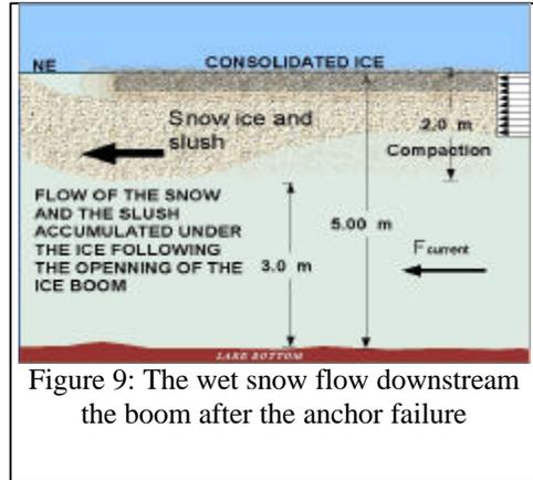
Figure 9: The wet snow flow downstream the boom after the anchor failure
