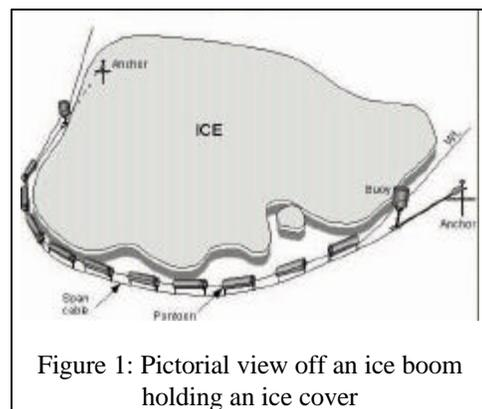
Figure 1: Pictorial view off an ice boom holding an ice cover
