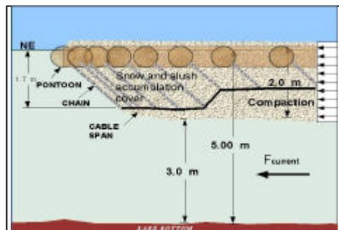
Figure 8: The wet snow retention by the boom.
