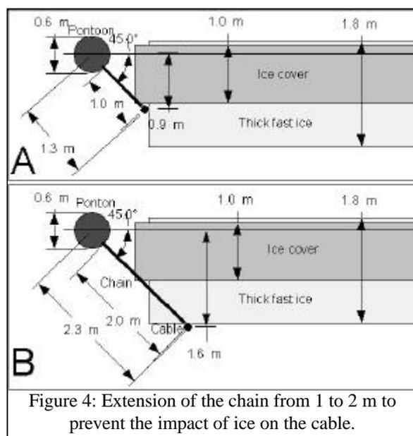
Figure 4: Extension of the chain from 1 to 2 m to prevent the impact of ice on the cable.
