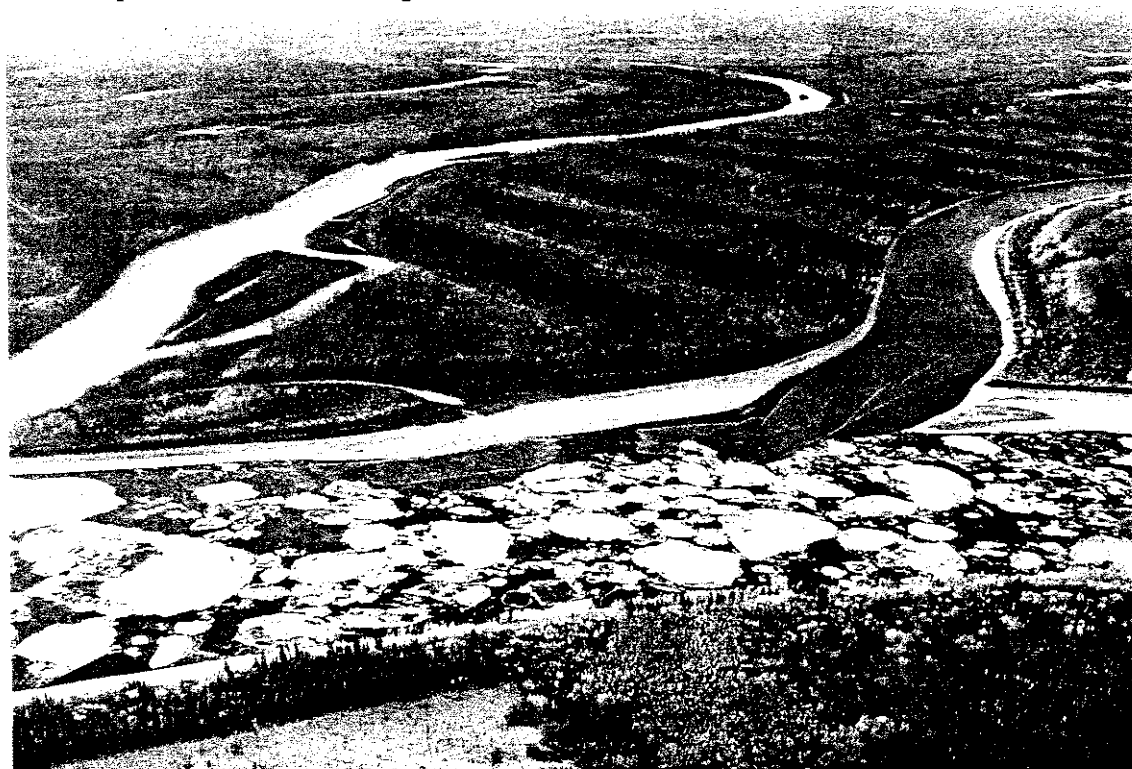
Figure 1 Ice floes and large rafts arriving at the head of an advancing ice cover
